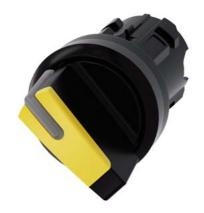
Selector switch, illuminable, 22 mm, round, plastic, yellow, selector switch, short, 2 switch positions O<I, momentary contact type, Actuating angle 45°, 10:30h/12h, with laser labeling, inscription or symbol Customer-specific selection with SIRIUS ACT configurator (CIN)
