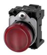
Indicator lights, 22 mm, round, plastic, red, lens, smooth, with holder, LED module, with integrated LED 24 V AC/DC, spring-type terminal, with laser labeling, lower case
