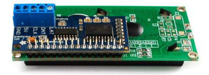
Make sure that as you solder the first pin, the backpack PCB isn't leaning against the LCD, where the terminal blocks could short against some components. You can put some electrical tape or foam tape behind to avoid this if you think it could be an issue.
