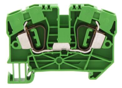
Feed-through terminal, Tension-spring connection, Mounting type: Mounting rail TS 35/7.5, Rated cross-section: 6 mm<sup>2</sup>, Width: 8.1 mm, Colour: Green
