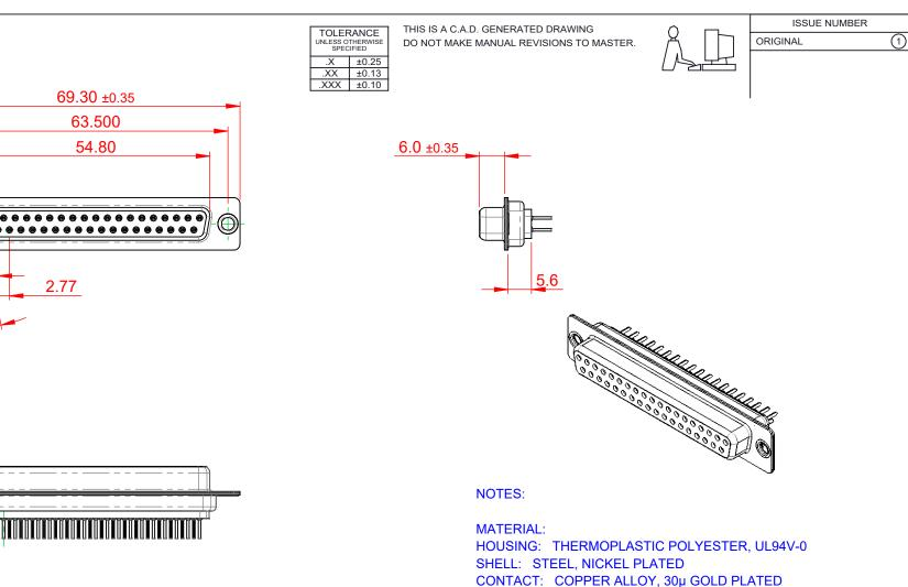
OPERATING TEMPERATURE: -55°C to +85°C CURRENT RATING: 3A PER CONTACT CONTACT RESISTANCE: 25mQ MAX.
