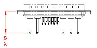
POWER/CO-AX CONTACT RATING:10A (CURRENT)(IF PRESENT)SIGNAL CONTACT CURRENT RATING:5A PER CONTACTSIGNAL CONTACT RESISTANCE:10mΩ MAX.INSULATOR RESISTANCE:5000MΩ min.DIELECTRIC5000MΩ min.
