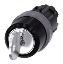
RONIS key-operated switch, 22 mm, round, plastic with metal front ring, lock number SB30, with 2 keys, 3 switch positions I>O<II, momentary contact on the left, latching on the right, actuating angle 2x45°, 10:30h/12h/13:30h, Key removal O+II, possible special locks: SB31, 421, 455, with laser labeling, upper case
