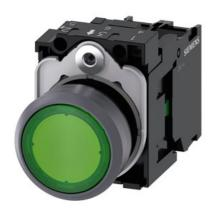
Illuminated pushbutton, 22 mm, round, plastic with metal front ring, green, pushbutton, flat, momentary contact type, with holder, 1NO, LED module with integrated LED 24 V AC/DC, screw terminal, with laser labeling, upper case and lower case, always upper case at beginning of line
