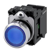
Illuminated pushbutton, 22 mm, round, metal, shiny, blue, pushbutton, flat, momentary contact type, with holder, 1NO, LED module with integrated LED 110 V AC, spring-type terminal, with laser labeling, lower case
