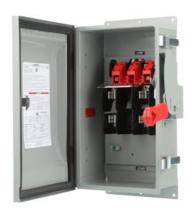
Siemens Low Voltage Circuit Protection Heavy Duty Safety Switches. Type: ENCLOSED, SAFETY SWITCH Std: UL V. Rating: 240V A. Rating: 60A Wattage: 2W No. Of Poles: 2P F. Rating: 60Hz Action: SINGLE THROW Material: 304SS Enclosure: TYPE 12. 2-3 point mounting holes. Insulation: YES O. Cycles: 10000 O. Temperature: (-20F-120F) AMBIENT TEMPERATURE Environmental Conditions: INDUSTRIAL
