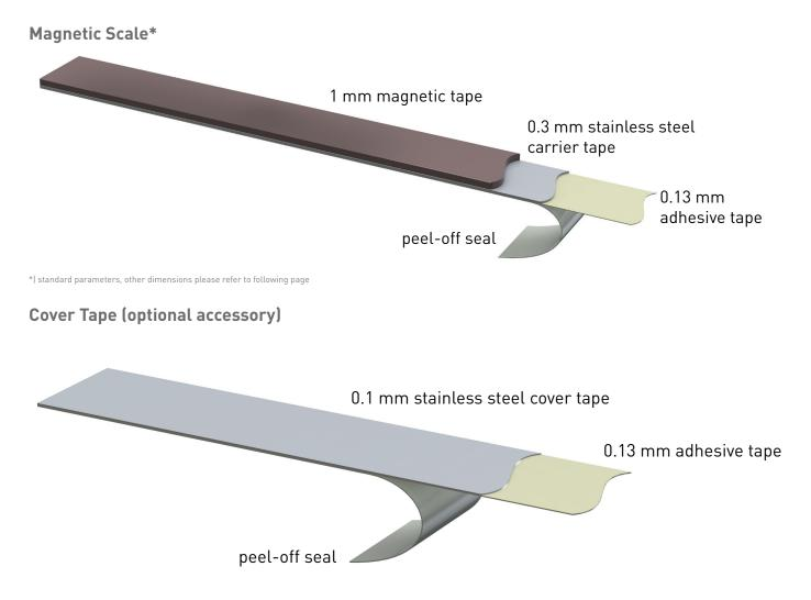
Due to mechanical characteristics of individual parts and applied manufacturing processes, the top surface of the magnetic component may show minimal surface changes. This has no negative impact on functionality.
