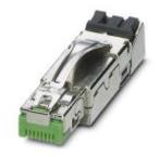
RJ45 connector, degree of protection: IP20, number of positions: 8, 10 Gbps, material: Zinc die-cast, connection method: IDC, connection cross section: AWG 26- 24, cable outlet: straight, High degree of resistance to vibration; 360° shielding; one-piece design; special tool-free assembly
