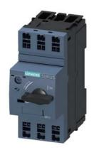
Special type Circuit breaker size S00 for motor protection, CLASS 10 A-release 10...16 A N-release 208 A Spring-type terminal Standard switching capacity Ambient temperature -50  $^{\circ}\text{C}$  500 switching cycles
