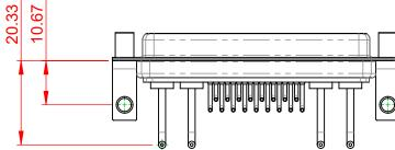
POWER/CO-AX CONTACT RATING: 10A (CURRENT) (IF PRESENT) SIGNAL CONTACT CURRENT RATING: 5A PER CONTACT
