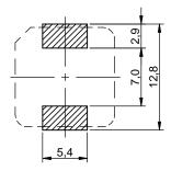
no sensitive traces underneath the component
