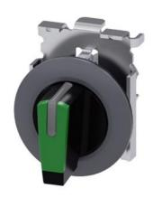
Selector switch, illuminable, 30 mm, round, Metal, matte, green, selector switch, short, front ring for flush installation, 3 switch positions I-O-II, latching, actuating angle 2x45°, 10:30h/12h/13:30h, Z=50-unit packaging
