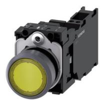
Illuminated pushbutton, 22 mm, round, plastic with metal front ring, yellow, pushbutton, flat, momentary contact type, with holder, 1 NO+1 NC, LED module with integrated LED 24 V AC/DC, spring-type terminal, with laser labeling, symbol number according to, ISO 7000 or IEC 60417
