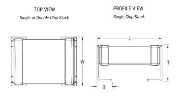
General Information Series KPS SMD Comm X7R Style Stacked Chip SMD, MLCC, Stacked, Single Chip, Temperature Description Stable Features Temperature Stable RoHS Yes Termination Tin AEC-Q200 No Component 410 mg Weight 2220-1 Chip Size 78 Weeks Shelf Life MSL 1
