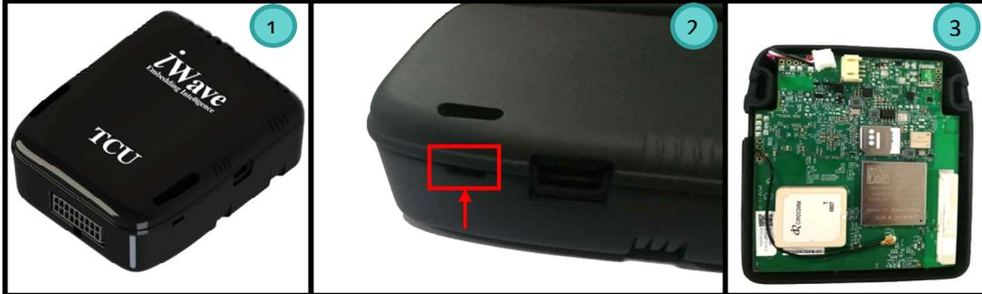
Figure 3 : Procedure to remove the enclosure
