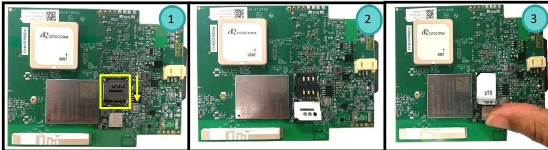
Figure 4 : SIM insertion procedure in Telematics control unit
