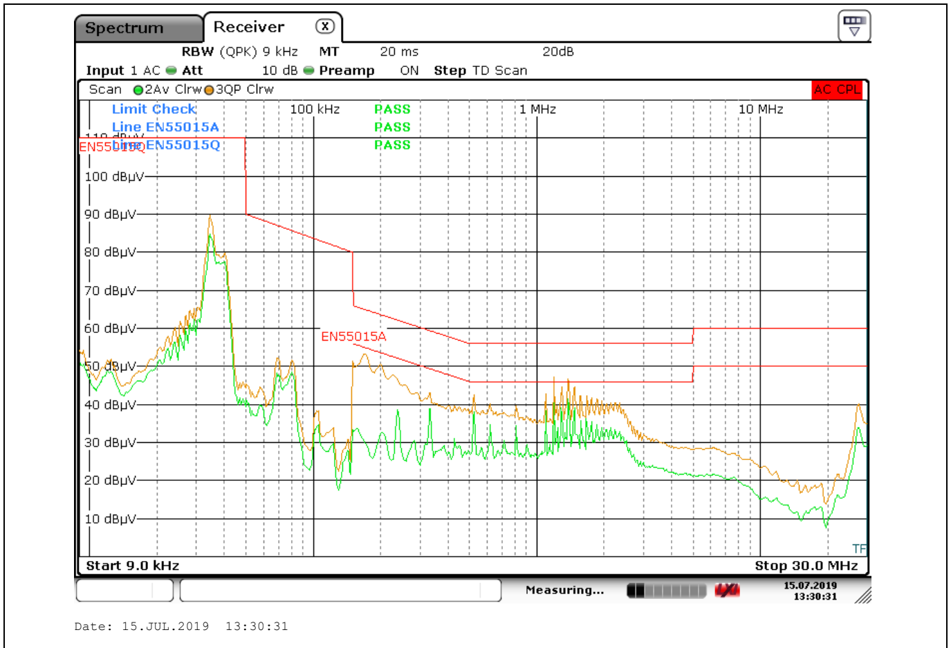
Figure 23 EMI spectrum at 250 V/50 Hz at full load (48 V LED, 3 A)
