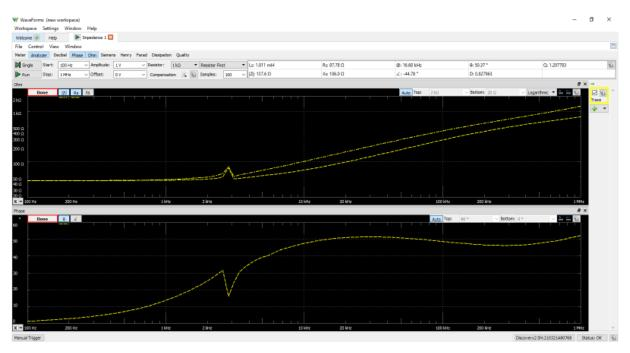
The Analog Discovery Studio can be used with WaveForms' "Impedance" instrument to view a wide variety of frequency response characteristics of a circuit under test. Input, Phase, Voltage, Current, Impedance, Admittance, Inductance, Factor, and Nyquist plots are all available. In addition, Custom plots can be used to present the results of a wide variety of different mathematical operations on buffered data.
