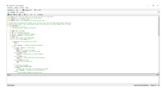
Each of WaveForms' instruments can be controlled through scripts within the WaveForms application itself. WaveForms' "Script" instrument allows the user to write and run javascript code that can control the rest of the application through an extensive API. This allows the user to configure and run many instruments at the same time, in an easily repeatable way.
