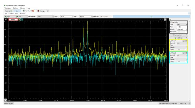
The Analog Discovery Studio can be used with WaveForms' "Spectrum" instrument to view the power of frequency-domain components of analog signals captured on the analog input channels.
