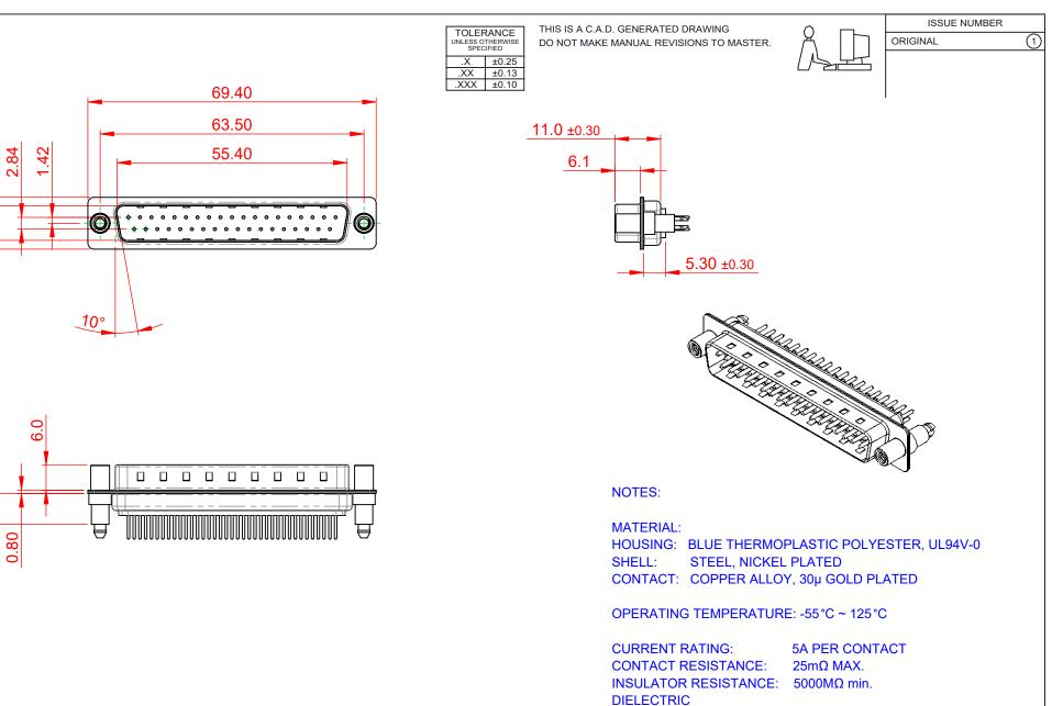
WITHSTANDING VOLTAGE: 1000V AC rms
