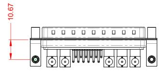
**OPERATING TEMPERATURE:** -55°C ~ 125°C 50Ω (IMPEDANCE) POWER/CO-AX CONTACT RATING: (IF PRESENT) SIGNAL CONTACT CURRENT RATING: 5A PER CONTACT SIGNAL CONTACT RESISTANCE:  $10m\Omega$  MAX. 5000MΩ min. **INSULATOR RESISTANCE:** DIELECTRIC
