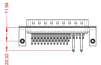
**OPERATING TEMPERATURE:** -55°C ~ 125°C POWER/CO-AX CONTACT RATING: (IF PRESENT) SIGNAL CONTACT CURRENT RATING: 5A PER CONTACT SIGNAL CONTACT RESISTANCE:  $10m\Omega$  MAX. **INSULATOR RESISTANCE:**
