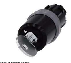
key-operated switch Siemens, 22 mm, round, plastic with metal front ring, lock no. LSG1, with 2 keys, 2 switch positions O-I, latching, actuating angle 90°, 10:30h/13:30h, key removal O, with laser labeling, upper case and lower case, always upper case at the beginning of the word
