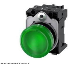
Indicator light, 22 mm, round, metal, shiny, green, lens, smooth, with holder, LED module with integrated LED 24 V AC/DC, screw terminal, with laser labeling, upper case and lower case, always upper case at beginning of line
