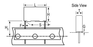
**General Information** Series F461 Dielectric Metallized Polypropylene Style Radial MKP, Pulse Features RoHS Yes Lead Wire Leads AEC-Q200 No Component 0.626 g Weight The Rated Voltage Decreases 2%/C Between +85C And +105C (1.25%/C For AC). ClimCat: Miscellaneous 55/105/56. Notes Series Replaced by R75.
