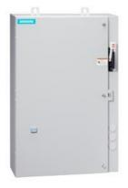
Non-reversing motor starter Size 0 Three phase full voltage Solid-state overload relay OLRelay amp range 0.75-3.4A 110-120/220-240VAC 60HZ coil Combination type 3Amp circuit breaker Encl NEMA type 4X 316 S-steel Water/dust tight noncorrosive Extra-wide enclosure
