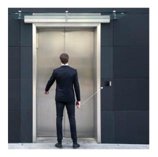
Angle detection makes it possible to determine on which side of the elevator a person is located. A building's entrance control system can use this information to only open the elevator's doors when the person is directly approaching them, increasing security.
