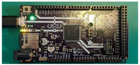
The Adafruit Grand Central M4 Express has a built-in SD card connected to the SPI bus, so no wiring or soldering is needed!
