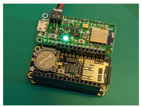
With all its built-in sensors and battery power, the Feather M4 Sense is great for data-logging projects. Stacking headers or FeatherWing Doublers need a little soldering but no custom wiring.
