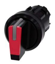
Selector switch, illuminable, 22 mm, round, plastic, red, selector switch, short, 3 switch positions I-O<II, left latching, right momentary contact type, actuating angle  $2x45^{\circ}$ , 10:30h/12h/13:30h Z=50-unit packaging
