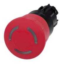
EMERGENCY STOP mushroom pushbutton, illuminable, 22 mm, round, plastic, red, 40 mm, positive latching, acc. to EN ISO 13850, rotate-to-unlatch, with laser labeling, upper case and lower case, always upper case at the beginning of the word
