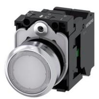
Illuminated pushbutton, 22 mm, round, Metal, shiny, white, pushbutton, flat, momentary contact type, with holder, 1NO, LED module with integrated LED 230 V AC, spring-type terminal, with laser labeling, upper case
