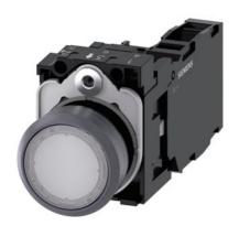
Illuminated pushbutton, 22 mm, round, plastic with metal front ring, white, pushbutton, flat, momentary contact type, with holder, 1 NO+1 NC, LED module with integrated LED 110 V AC, screw terminal, with laser labeling, symbol number according to, ISO 7000 or IEC 60417
