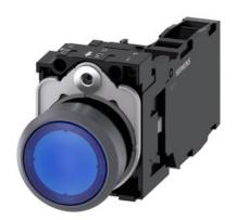
Illuminated pushbutton, 22 mm, round, plastic with metal front ring, blue, pushbutton, flat, momentary contact type, with holder, 1 NO+1 NC, LED module with integrated LED 230 V AC, screw terminal, with laser labeling, lower case
