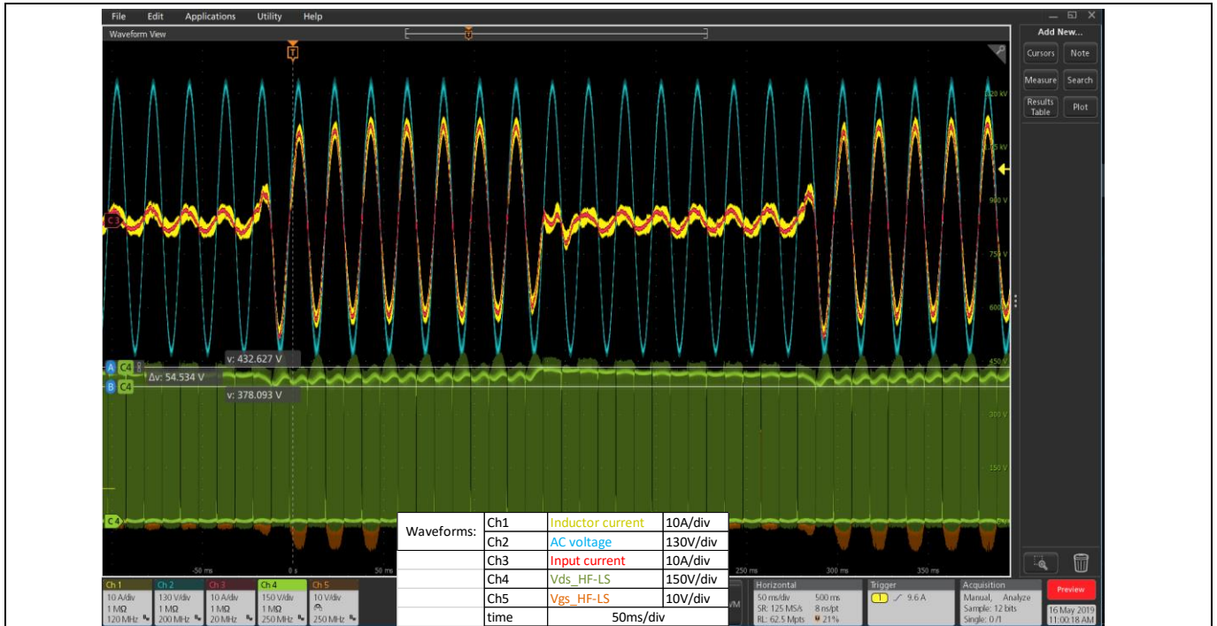
Figure 19 3.3 kW SiC totem-pole CCM PFC response for 10 percent to 90 percent load steps every 150 ms with 0.2 A/ \mu s current slope
