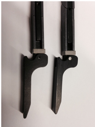
Left: Previous design with pin Right: New design with rivet
