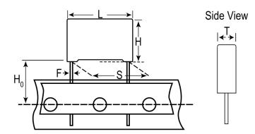
**General Information** Series R46 275 VAC Dielectric Metallized Polypropylene Style Radial Features EMI Safety RoHS Yes Lead Wire Leads Safety Class Х2 ENEC, UL, cUL, CQC Qualifications AEC-Q200 No THB Performance No Notes We Recommended To Use R46 @ 310 VAC.
