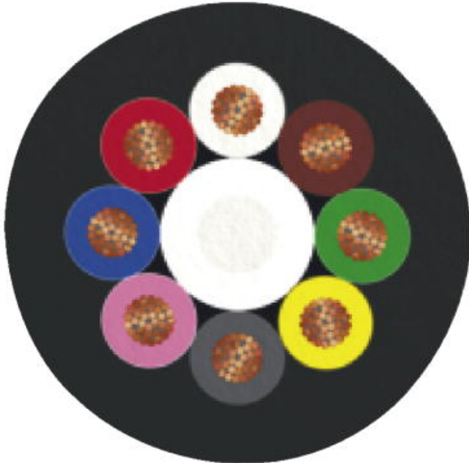
Cable cross section
