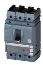
circuit breaker 3VA5 UL frame 250 breaking capacity class H 65kA @ 480 V 3-pole, line protection TM210, FTFM, In=175A overload protection Ir=175A fixed short-circuit protection Ii=10 x In UL489 SB (naval), 50 deg. cel. nut keeper kit on both sides
