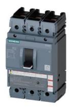
circuit breaker 3VA5 UL frame 250 breaking capacity class C 100kA @ 480 V 3-pole, line protection TM210, FTFM, In=200A overload protection Ir=200 A fixed short-circuit protection Ii=10 x In UL489 SB (naval), 50 deg. cel. nut keeper kit on both sides
