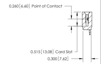
ACAD REFERENCE NO. 745 Series Ultra-Mate Card Edge Connector - Press Fit DRAWN: J.LEE Part Number: 745-045-520-101 CHECKED: SCALE: **EDAC INC** THESE DRAWINGS AND SPECIFICATIONS ARE THE PROPERTY OF EDAC INC.,AND TORONTO, ONTARIO SHALL NOT BE REPRODUCED, OR COPIED DRAWING NUMBER CANADA OR USED AS THE BASIS FOR THE 745-ENG MASTER MANUFACTURE OR SALE OF APPARATUS YOUR CONNECTION TO QUALITY & SERVICE WITHOUT WRITTEN PERMISSION.
