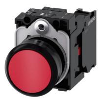
Pushbutton, 22 mm, round, plastic, red, pushbutton, flat, momentary contact type, with holder 1 NC, screw terminal, with laser labeling, symbol number according to, ISO 7000 or IEC 60417
