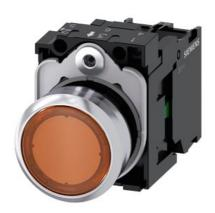
Illuminated pushbutton, 22 mm, round, metal, shiny, amber, pushbutton, flat, momentary contact type, with holder, 1NO, LED module with integrated LED 110 V AC, screw terminal, with laser labeling, upper case and lower case, Always upper case at the beginning of the word
