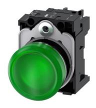
Indicator lights, 22 mm, round, metal, shiny, green, lens, smooth, with holder, LED module with integrated LED 110 V AC, screw terminal, with laser labeling, upper case and lower case, always upper case at the beginning of the word
