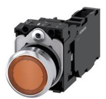
Illuminated pushbutton, 22 mm, round, metal, shiny, amber, pushbutton, flat, momentary contact type, with holder, 1 NO+1 NC, LED module with integrated LED 230 V AC, screw terminal, with laser labeling, inscription or symbol Customer-specific selection with SIRIUS ACT configurator (CIN)
