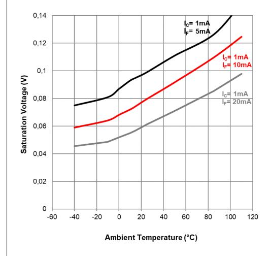
Testcondition: I<sub>E</sub>= 5mA, Normalized to 25°C
