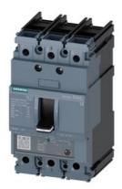
circuit breaker 3VA5 UL frame 125 breaking capacity class M 35kA @ 480 V 3-pole, line protection TM230, FTAM, In=25A overload protection Ir=25A fixed short-circuit protection Ii=6...12 x In UL489 SB (naval), 50 deg. cel. nut keeper kit on both sides
