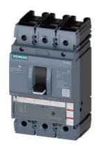
circuit breaker 3VA5 UL frame 250 3-pole, starter protection TM120M, AM, In=200A without overload protection short-circuit protection Ii=3...6 x In nut keeper kit on both sides
