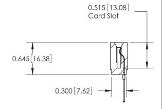
737 Series Ultra-Mate Card Edge Connector - Press Fit ACAD REFERENCE @TION - ACAD REFERENCE
